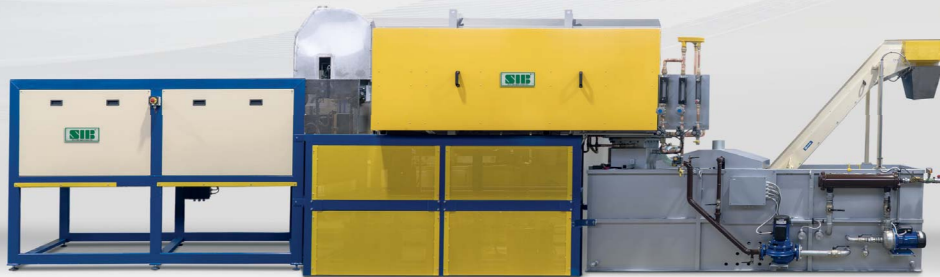
CONTINUOUS CARBURIZING AND HARDENING LINE FOR MEDIUM / SMALL METAL PARTS
